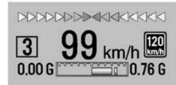
**Format Four:** This display gives the speedometer reading (in English or metric units), transmission positions (for automatic transmission vehicles only), Shift Timing Light Position and lateral acceleration (G) indicators.
