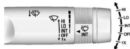
The window wiper/washer lever is on the right side of the steering column. With the ignition in ACC/ACCESSORY or ON/RUN, move the window wiper lever to select the wiper speed.
