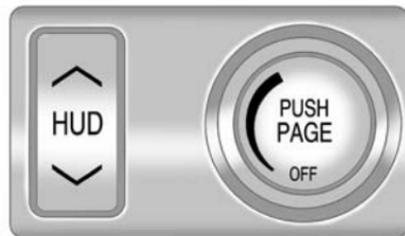
The HUD control is located to the right of the steering wheel.
