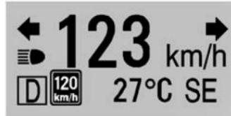
**Format One:** This display gives the speedometer reading (in English or metric units), indicator signal indication, main beam indication, transmission positions, speed alert, and outside air temperature.
