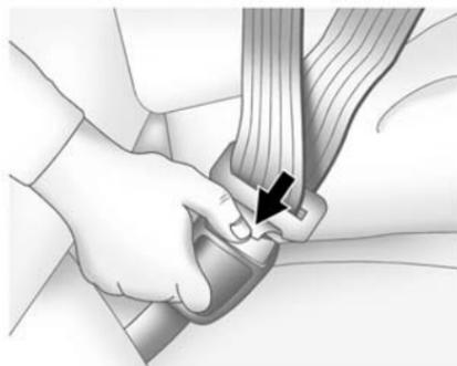
To unlatch the belt, push the button on the buckle. The belt should return to its stowed position.
