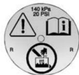
3. Cover the radiator cap with a thick cloth and turn it slowly counterclockwise and remove.
