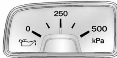
For vehicles with the oil pressure gauge, it is located in front of the gear lever, and shows the engine oil pressure in kPa (kilopascals).
