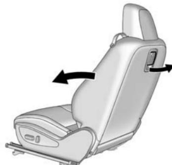
To access the rear seats, pull up on the latch on the rear of the driver or front passenger seatback. Fold the backrest forward.
