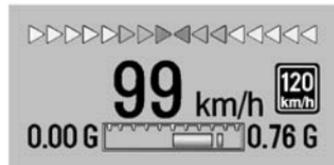
Vehicles equipped with a Head-Up Display (HUD) may also have shift timing lights across the top of the display. As you approach a shift point, the rows of lights grow closer together. The transmission should be shifted before the lights come together in the middle of the display. If the lights begin flashing, you have exceeded the shift point. Shift immediately.
