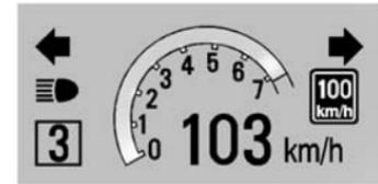
**Format Three:** This display includes the information in Format One along with a circular tachometer, but without outside air temperature.
