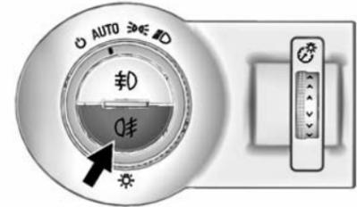
The rear fog lamp button is on the exterior lamp control on the outboard side of the steering wheel.
