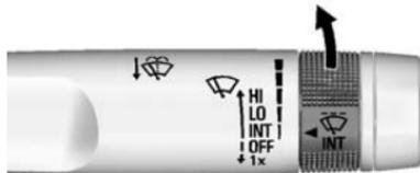
**INT (Intermittent Wipes):** Move the lever up to INT for intermittent wipes, then turn the
