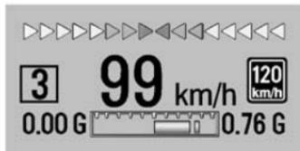
Vehicles equipped with a Head-Up Display (HUD) also have shift timing lights across the top of the display. As you approach a shift point, the rows of lights grow closer together. The transmission should be shifted
