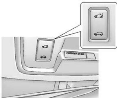
**Open/Close:** Press and hold the rear or front of the switch to open or close the sunroof.
