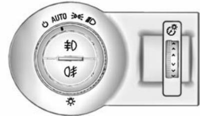
The exterior lamp control is on the instrument panel, on the outboard side of the steering wheel.
