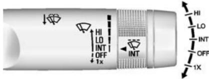
The windscreen wiper/washer lever is on the right side of the steering column. With the ignition in ACC/ACCESSORY or ON/RUN, move the windscreen wiper lever to select the wiper speed.
