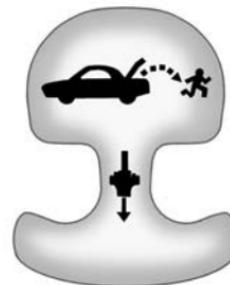
There is an emergency boot release handle inside the boot on the liner, near the boot latch. On some vehicles, the release handle can be accessed by folding the rear seatback down. See *Rear Seats on page 3-6*.
