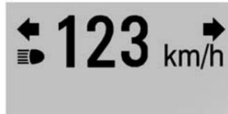
**Format Two:** This display includes the information in Format One without the transmission information, speed alert, and the outside air temperature.
