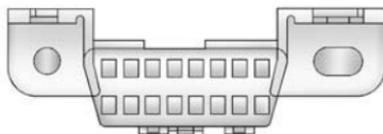
The DLC is under the instrument panel to the left of the steering wheel. See your dealer if assistance is needed.
