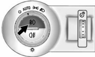
The front fog lamps button is on the exterior lamp control, on the outboard side of the steering wheel.
