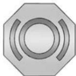
The brake/hydraulic clutch fluid reservoir cap has this symbol on it. The common hydraulic clutch and brake master cylinder fluid reservoir is filled with DOT 3 brake fluid as indicated on the reservoir cap. See *Engine Compartment Overview on page 10-5* for reservoir location.
