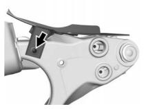
Install the control arm deflector to the upper duct using the screw. Do not tighten at this time.
