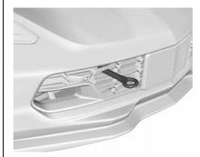
The front tow eye socket is accessible through the grille opening.
