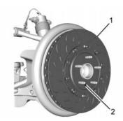
Install the rotor (1) with the fastener (2). Torque to 10 N•m (89 lb inch).
