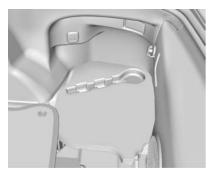
The tow eye is located underneath the load floor, near the spare tyre or the compressor kit, if equipped. Carefully open the cover in the fascia by using the small notch that conceals the tow eye socket.
