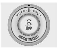
The TCS/StabiliTrak button is on the centre console.
