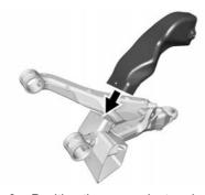
Position the upper duct and snap it into the tabs of the front and rear airbox assembly.
