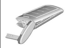
Use the oval base of the key blade to separate the two halves of the transmitter.
