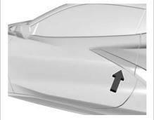
For Keyless Access, hold the remote key within 1 m (3 ft) of the door handle. Grip and press the door handle touchpad. See *Remote Key Operation*  $\Rightarrow$  8. This feature can be programmed. To view available settings from the infotainment screen, touch Settings > Vehicle > Remote Lock, Unlock, Start.
