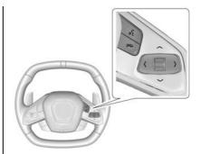
Press  $\leq$  or > to access the cluster applications. Use the thumbwheel to scroll
