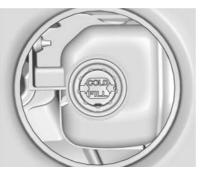
When the engine is cold, the coolant level should be at the COLD FILL indicator in the coolant surge tank.
