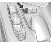
The TCS/StabiliTrak/ESC button is on the centre console.
