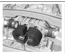
Remove the air cleaner/filter(s) (top image LT2 engine) (bottom image LT6 engine).
