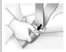
To unlatch the belt, push the button on the buckle. The belt should return to its stowed position.
