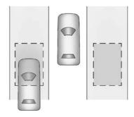
The SBZA sensor covers a zone approximately one lane over from both sides of the vehicle, or approximately 3.5 m (11 ft). The height of the zone is approximately between 0.5 m (1.5 ft) and 2 m (6 ft) off the ground. This zone starts at approximately the middle of the vehicle and goes back 5 m (16 ft).
