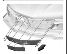
For Z06 vehicles only, remove the front number plate and bracket (if installed) and remove the front aero covers before track use. See your retailer for complete procedure.
