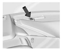
If equipped, the indicator light, on the instrument panel near the windscreen, indicates the status of the system.
