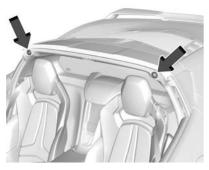
5. Position the rear edge of the roof panel next to the weatherstrip on the back of the roof opening. Then align and fit the pins at the rear of the roof panel inside the openings in the rear overhead weatherstrip. Gently lower the front edge of the roof panel to the front of the roof opening.
