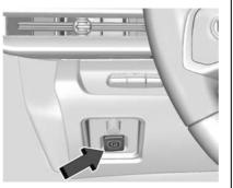
The Electric Parking Brake (EPB) can always be applied, even if the vehicle is switched off. In case of insufficient electrical power, the EPB cannot be applied or released. To prevent draining the battery, avoid unnecessary repeated cycles of the EPB.
