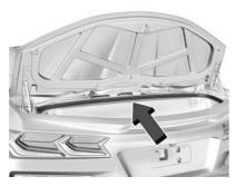
Use the pull cup to close the hatch/trunk with light force until the power latch feature activates. The hatch/boot will close the rest of the way and latch automatically.
