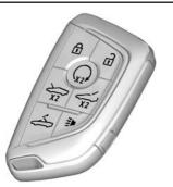
1 : Press to lock both doors and the fuel door. The indicators may flash and/or the horn may sound on the second press to indicate locking. To view available settings from the infotainment screen, touch Settings > Vehicle > Remote Lock, Unlock, Start.
