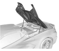
5. Hold عنه until the tonneau cover is completely opened. The turn signals will flash once.
