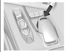
To activate My Mode, Weather, Tour, Sport and Track Mode, turn the Driver Mode Control (DMC) knob on the center console to make a mode selection. When a mode is selected, an indicator will illuminate in the instrument cluster and remain illuminated.
