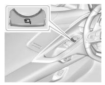
If equipped, press <sup>E</sup>₄ to power fold the mirrors. Press <sup>E</sup>₄ again to unfold.
