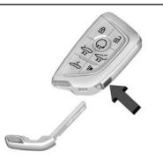
Press the button on the side of the remote key and pull the mechanical key out. Never pull the mechanical key out without pressing the button.
